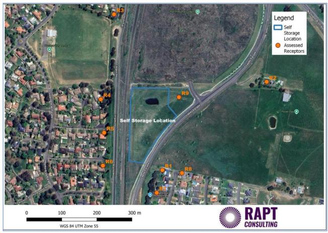
Figure 13 - site plan indicated noise sensitive receptors assessed under the submitted acoustic assessment
