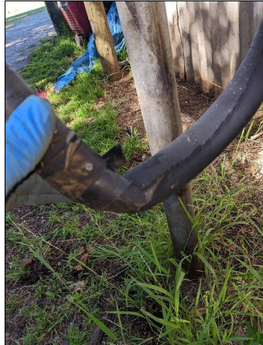
Kinks identified in the fuel pump hose
