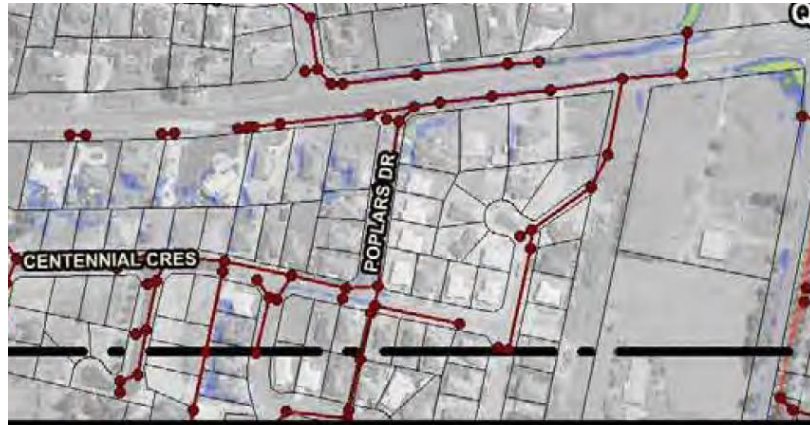
Figure 3 - 5% AEP storm event - pits starting to surcharge in Poplars
