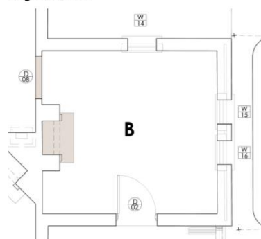
Figure 5.19 Former gardener's office and interps space: The interpretation display should always respect the characteristics of the room and allow the heritage architectural values to be interpreted as well. Low displays under windows will allow windows to be appreciated. Also noted here are the reconstruction of the lost fireplace surrounds and the potential for reinstating a door that may be indicated by the cracking patterns – Adaptive Architects 2021
