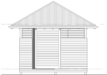
Figure 9.2 A compatible toilet block for a Victorian era park needs to interpret some of the Victorian era characteristics even if the materials are modern. Then using colours and materials that blend with the landscape the toilets will not intrude on the character of the significant landscape – Adaptive Architects 2021 Using this strategy of determining what is significant, and what level of change can be accommodated, we can then have a more consistent approach in our policy development. We can encourage change, while still preserving significance.
